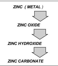
metal underneath. The corrosion rate of the overall system depends on the rate of zinc carbonate erosion or dissolution. Very basic or very acidic solutions can dissolve this layer extremely rapidly. The corrosion rate changes most rapidly in the low pH atmosphere because acidic solutions quickly dissolve the zinc carbonate layer. This is seen in the corrosion rate chart of Fig. 4. A high pH atmosphere can also shorten the life of the zinc coating.
