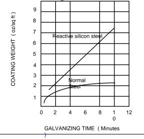
main concern with reactive steel galvanized coatings is the thickness of the coating. If the coating is too thick it may become brittle and will be susceptible to applied stresses that may separate the galvanized coating from the steel underneath. Knowing the silicon and phosphorous content is very important to producing a quality galvanized coating.
